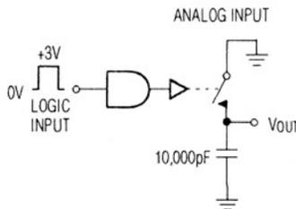
Figure 2. Charge Injection
