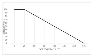
The case temperature is to be used for the definition of the applied power limit
