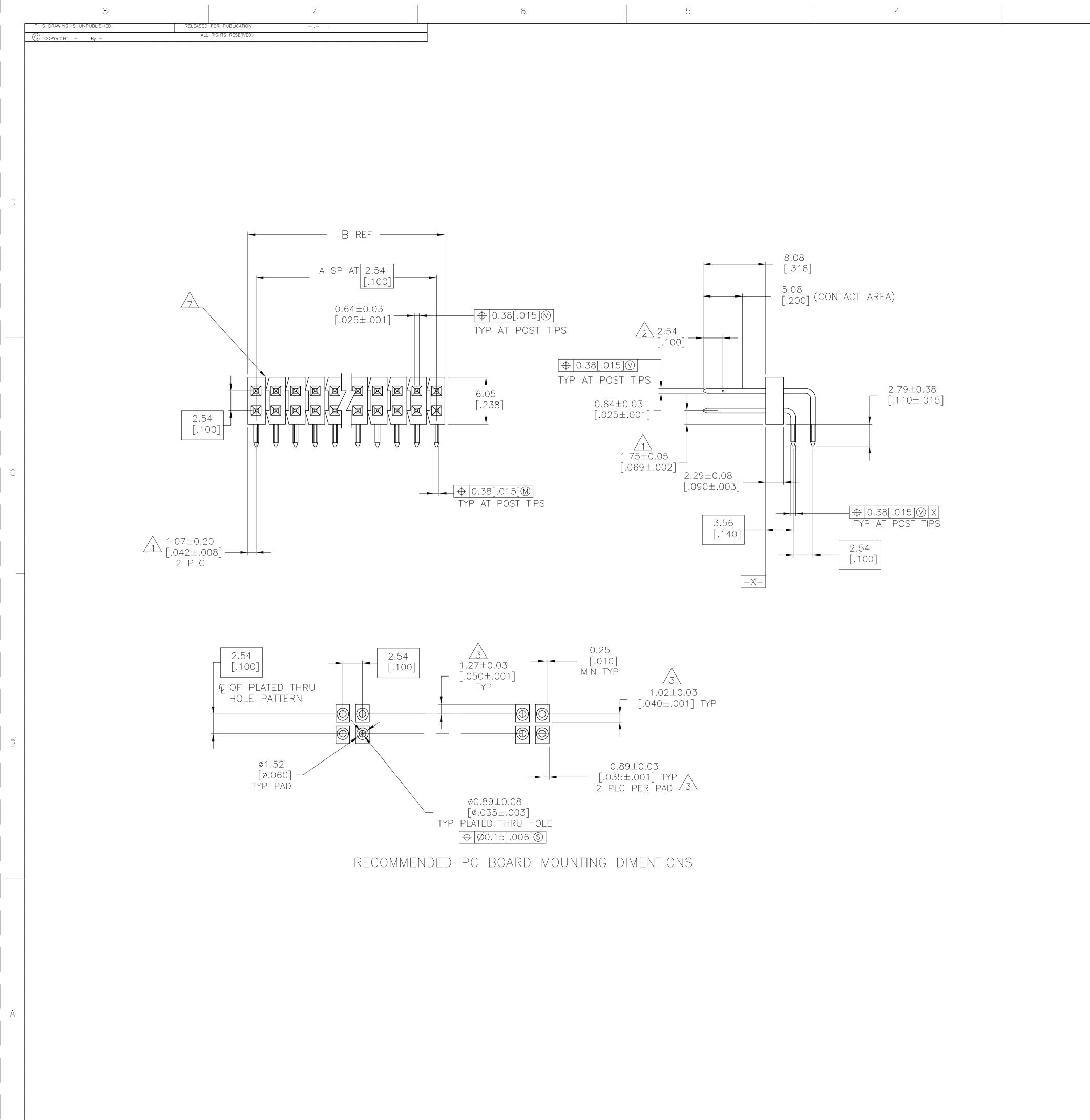
THE NOTED DIMENSIONS APPLY AT THE INTERSECTION OF THE POST AND HOUSING POINT OF MEASUREMENT FOR PLATING THICKNESS. DIMENSIONS NOTED ARE FOR USE WITH A STENCIL FOR 1.57±0.20[.062±.008] THICK PRINTED CIRCUIT BOARD SOLDER STENCIL THICKNESS =  $0.25\pm0.03[.010\pm.001]$ .000381 [.000015] GOLD IN THE CONTACT AREA.
