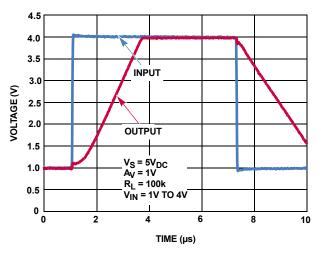
FIGURE 58. CHARACTERIZED LARGE SIGNAL STEP RESPONSE (3V)
