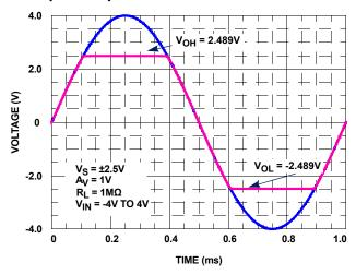
FIGURE 63. SIMULATED NO PHASE INVERSION,  $V_{\mbox{OH}}$  and  $V_{\mbox{OL}}$
