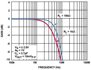
FIGURE 28. GAIN vs FREQUENCY vs  $R_L$ ,  $V_S = 5.0V$
