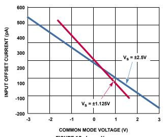
FIGURE 12.  $I_{OS}$  vs  $V_{CM}$
