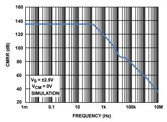
FIGURE 56. CHARACTERIZED CMRR vs FREQUENCY
