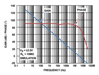
FIGURE 52. CHARACTERIZED OPEN-LOOP GAIN, PHASE vs FREQUENCY
