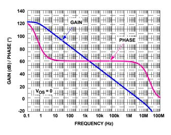
FIGURE 53. SIMULATED OPEN-LOOP GAIN, PHASE vs FREQUENCY
