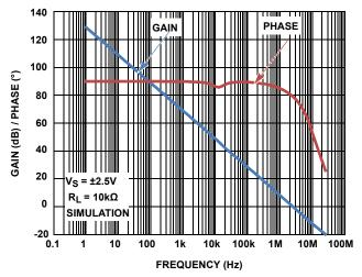
FIGURE 25. OPEN LOOP GAIN AND PHASE,  $R_L = 10k$
