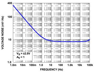
FIGURE 51. SIMULATED INPUT NOISE VOLTAGE
