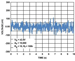
FIGURE 22. INPUT NOISE VOLTAGE 0.1Hz TO 10Hz
