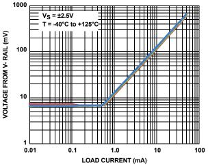
FIGURE 18. OUTPUT LOW OVERHEAD VOLTAGE vs LOAD CURRENT
