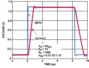
FIGURE 40. LARGE SIGNAL STEP RESPONSE (1V)
