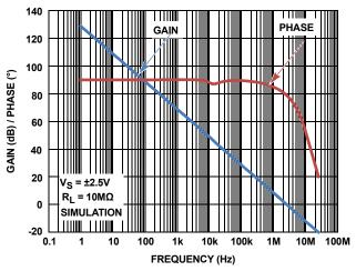
FIGURE 24. OPEN LOOP GAIN AND PHASE,  $R_L = 10M$
