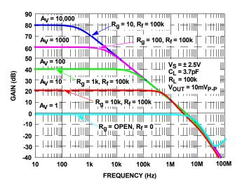
FIGURE 55. SIMULATED CLOSED-LOOP GAIN vs FREQUENCY
