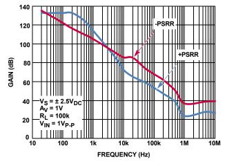
FIGURE 36. PSRR vs FREQUENCY,  $V_S = 5V$
