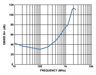
FIGURE 33. EMIRR AT IN+ PIN vs FREQUENCY
