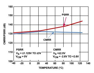
FIGURE 15. CMRR and PSRR vs TEMPERATURE
