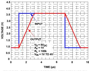
FIGURE 59. SIMULATED LARGE SIGNAL STEP RESPONSE (3V)
