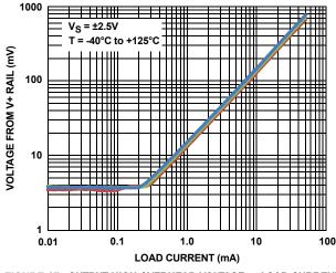
FIGURE 17. OUTPUT HIGH OVERHEAD VOLTAGE vs LOAD CURRENT
