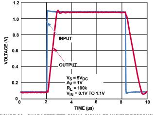
FIGURE 60. CHARACTERIZED SMALL-SIGNAL TRANSIENT RESPONSE
