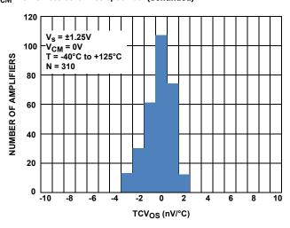
FIGURE 8.  $TCV_{OS}$  HISTOGRAM  $V_S = 2.5V$
