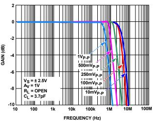
FIGURE 30. GAIN vs FREQUENCY vs Vout
