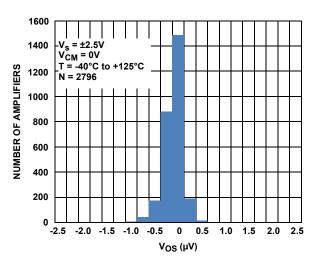
FIGURE 5.  $V_{OS}$  HISTOGRAM  $V_S = 5V$
