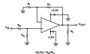
FIGURE 44. CIRCUIT IMPLEMENTATION FOR REDUCING INPUT BIAS CURRENTS
