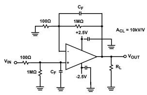
FIGURE 47. HIGH GAIN, PRECISION DC-COUPLED AMPLIFIER
