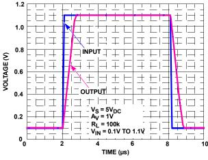
FIGURE 61. SIMULATED SMALL-SIGNAL TRANSIENT RESPONSE
