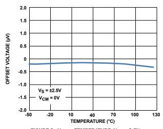
FIGURE 3.  $V_{OS}$  vs TEMPERATURE,  $V_S = \pm 2.5V$
