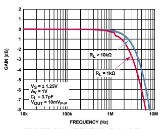
FIGURE 27. GAIN vs FREQUENCY vs  $R_{L}$ ,  $V_{S} = 2.5V$
