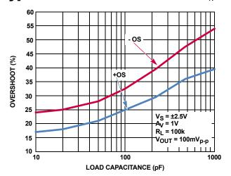
FIGURE 42. SMALL SIGNAL OVERSHOOT vs LOAD CAPACITANCE,  $VS = \pm 2.5V$
