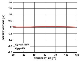
FIGURE 4.  $V_{OS}$  vs TEMPERATURE,  $V_S = \pm 1.125V$
