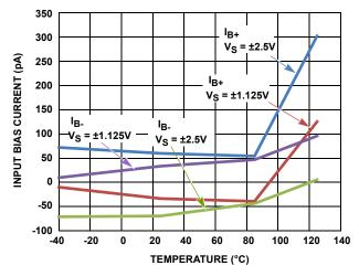
FIGURE 13. IB vs TEMPERATURE
