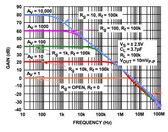
FIGURE 54. CHARACTERIZED CLOSED-LOOP GAIN vs FREQUENCY
