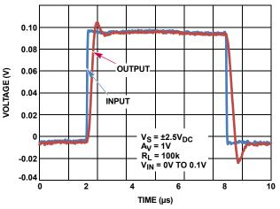
FIGURE 41. SMALL SIGNAL STEP RESPONSE (100mV)
