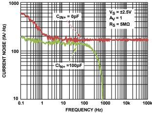
FIGURE 23. INPUT NOISE CURRENT DENSITY vs FREQUENCY
