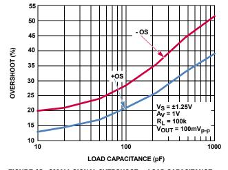
FIGURE 43. SMALL SIGNAL OVERSHOOT vs LOAD CAPACITANCE,  $V_S = \pm 1.25 V$
