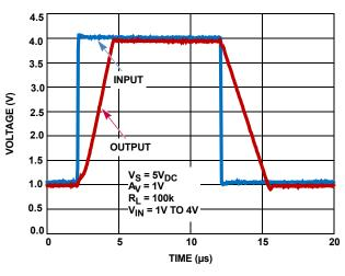
FIGURE 39. LARGE SIGNAL STEP RESPONSE (3V)
