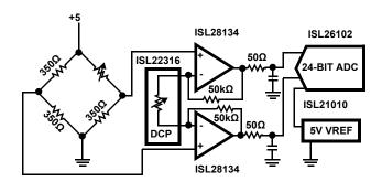
FIGURE 1. PRECISION WEIGH SCALE / STRAIN GAUGE
