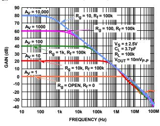
FIGURE 26. FREQUENCY RESPONSE vs CLOSED LOOP GAIN
