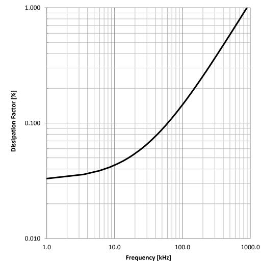
Test Equipment: E4991A or equivalent
