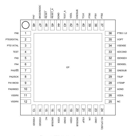
Figure 3. MM912\_637 pin connections
