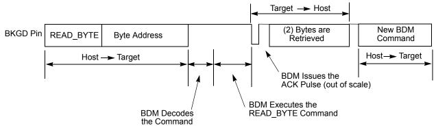
Figure 87. Handshake protocol at command level
