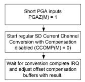
Figure 38. Current channel offset compensation sequence
