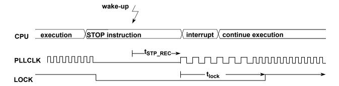
Figure 95. Stop mode using PLLCLK as bus clock
