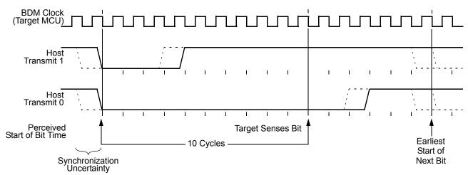
Figure 83. BDM host-to-target serial bit timing
