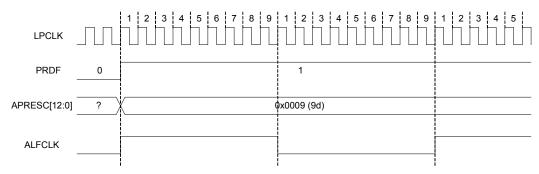
Figure 25. ALFCLK after calibration
