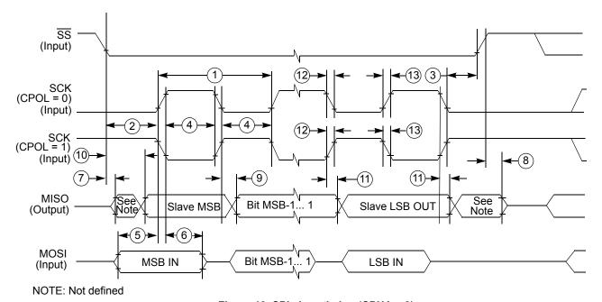
Figure 10. SPI slave timing (CPHA = 0)
