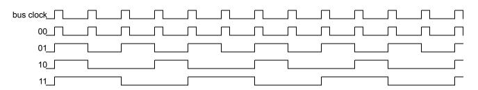
Figure 116. Interface clock waveforms for various D2DCLKDIV encoding
