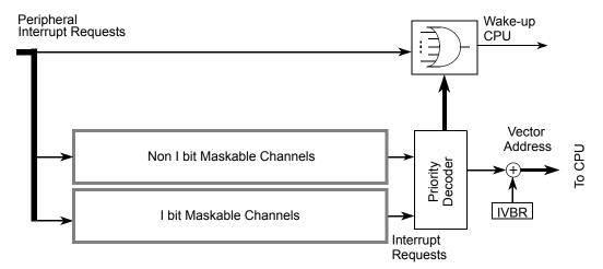
Figure 54. 9S12I128PIMV1 block diagram
