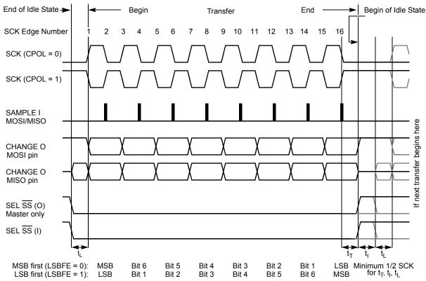
t<sub>L</sub> = Minimum leading time before the first SCK edge, not required for back-to-back transfers
