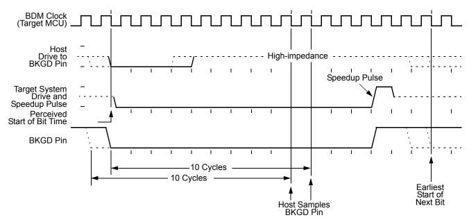
Figure 85. BDM target-to-host serial bit timing (logic 0)
