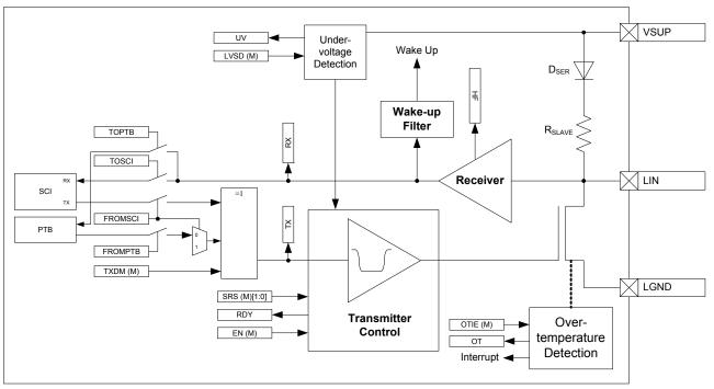
Figure 44. LIN module block diagram
