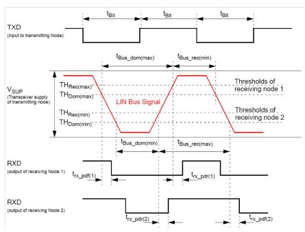
Figure 45. Definition of LIN bus timing parameters
