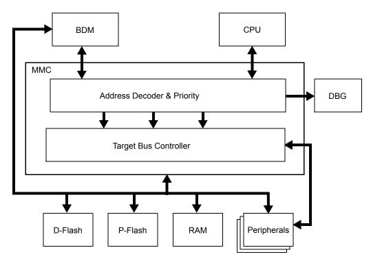
Figure 55. S12PMMC block diagram
