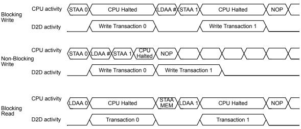
Figure 117. Blocking and non-blocking transfers.
