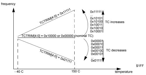
Figure 93. Influence of TCTRIM[4:0] on the temperature coefficient
