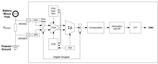
Figure 29. Current measurement channel
