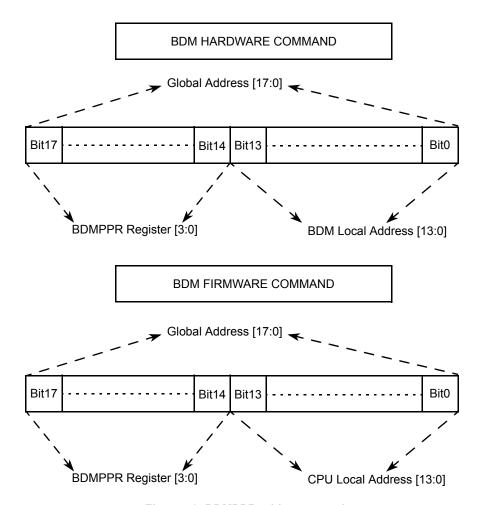
Figure 59. BDMPPR address mapping
