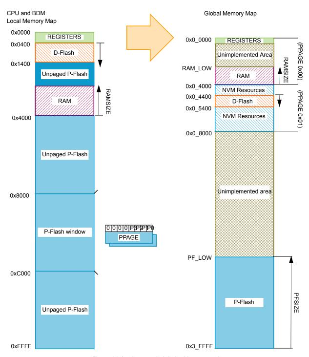
Figure 61. Implemented global address mapping
