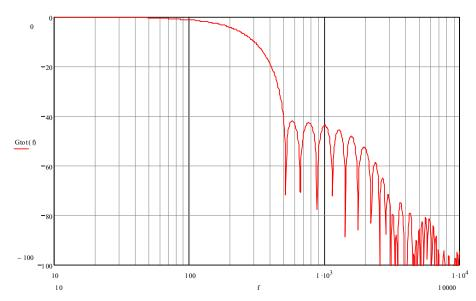
Figure 35. Typical total filter response Sinc3 (D=128), LP filter (FIR type with 15 coefficients used)
