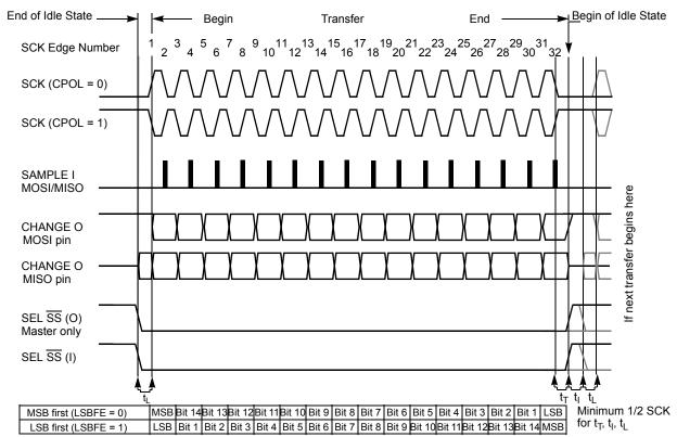
t<sub>I</sub> = Minimum leading time before the first SCK edge, not required for back-to-back transfers
