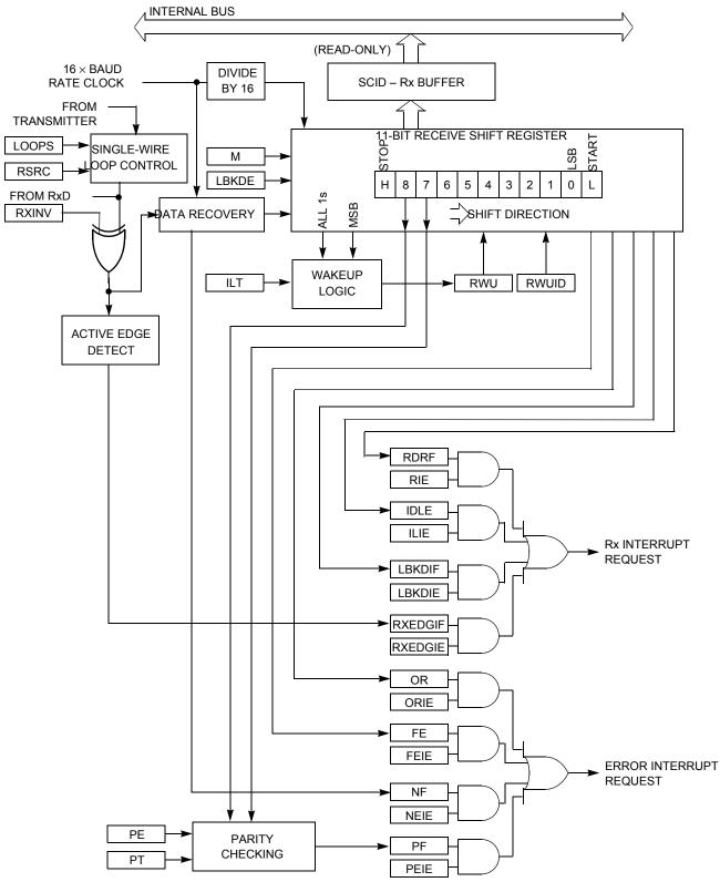
Figure 47. SCI receiver block diagram
