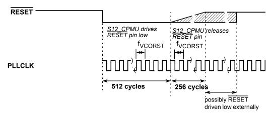
Figure 100. RESET timing
