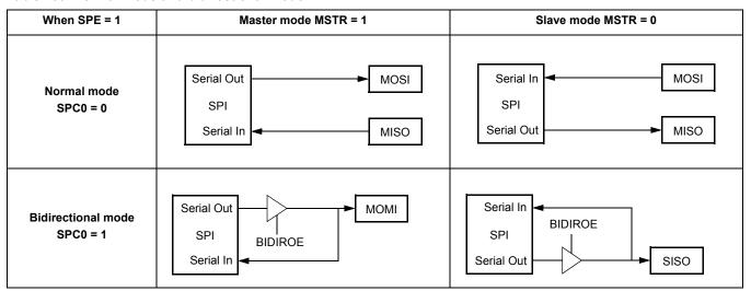
The direction of each serial I/O pin depends on the BIDIROE bit. If the pin is configured as an output, serial data from the shift register is driven out on the pin. The same pin is also the serial input to the shift register.
