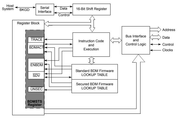
Figure 81. BDM block diagram
