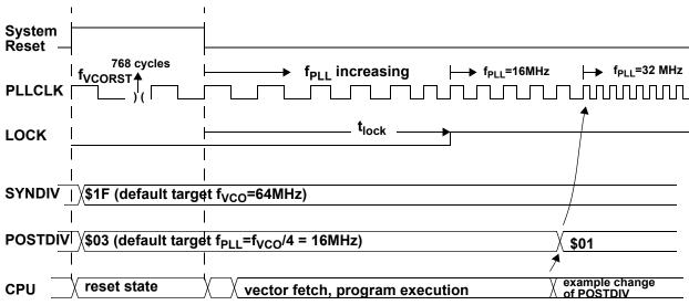
Figure 94. Startup of clock system after reset
