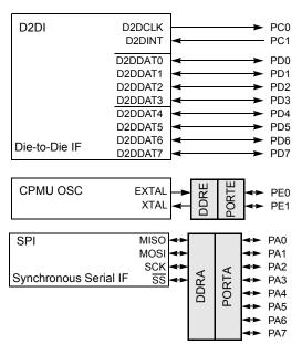
Figure 52. Port integration module - block diagram
