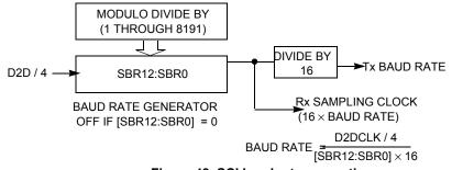
Figure 48. SCI baud rate generation
