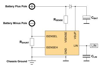
Figure 12. Typical IBS application (device GND = chassis GND)
