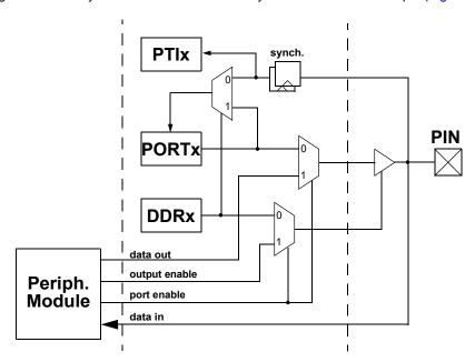
Figure 53. Illustration of I/O pin functionality
