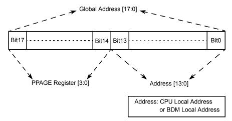
Figure 58. PPAGE address mapping
