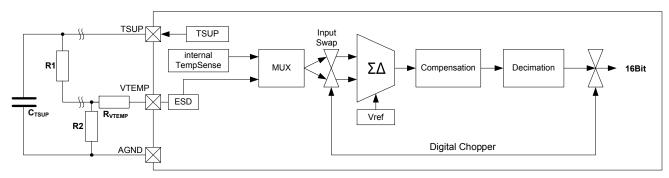
Figure 31. Temperature measurement channel
