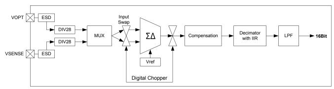
Figure 30. Voltage Measurement Channel
