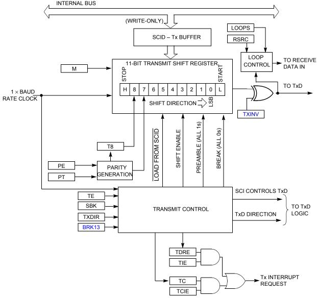
Figure 46. SCI transmitter block diagram
