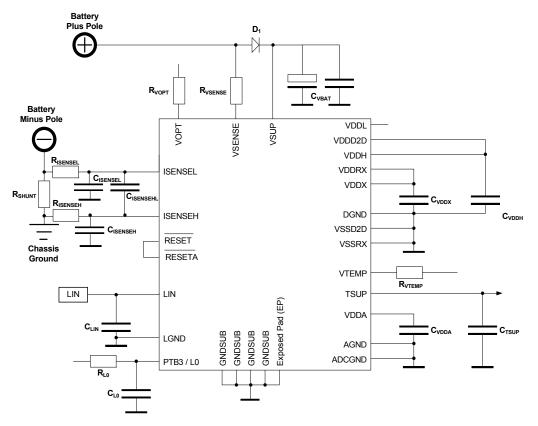
Note: Module GND connected to Battery Minus or Chassis Ground – based on configuration.
