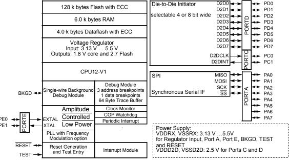
Figure 50. MC9S12I128 block diagram
