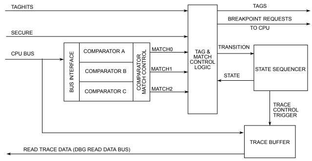
Figure 63. Debug module block diagram
