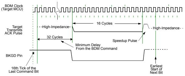
Figure 86. Target acknowledge pulse (ACK)
