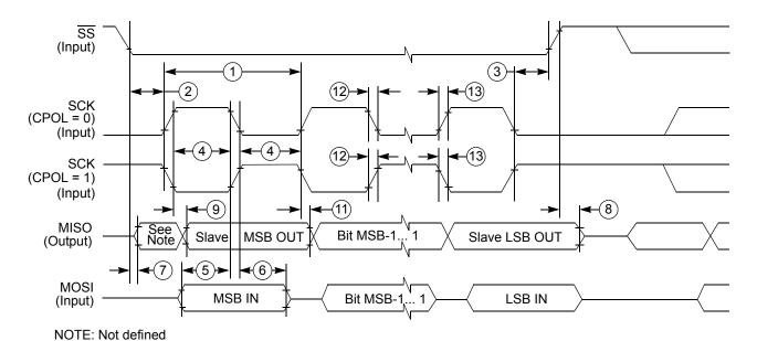
Figure 11. SPI slave timing (CPHA = 1)
