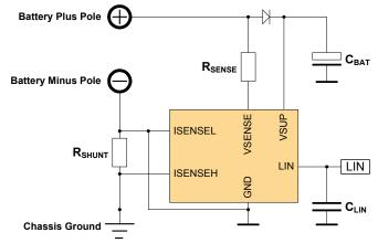
Figure 13. Typical IBS application (device GND = battery minus)
