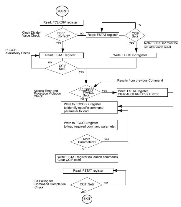
Figure 112. Generic flash command write sequence flowchart
