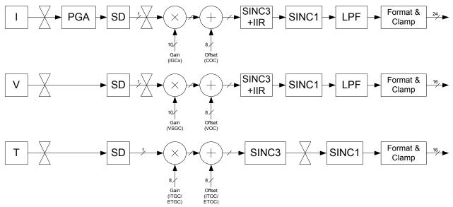
Figure 32. Simplified measurement channel
