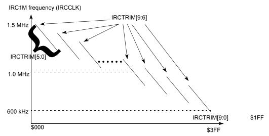
Figure 92. IRC1M frequency trimming diagram
