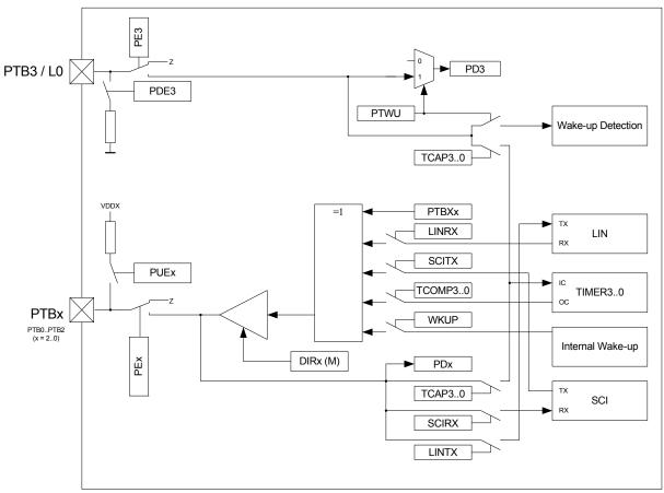
Figure 42. General purpose I/O - block diagram
