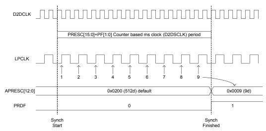
Figure 24. ALF clock calibration procedure during normal mode
