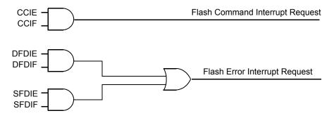
Figure 113. Flash module interrupts implementation
