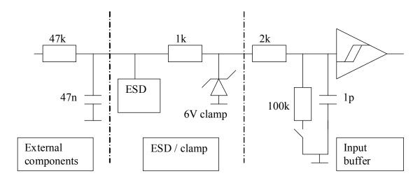
Figure 43. L0 / PTB3 input structure (typical values indicated)
