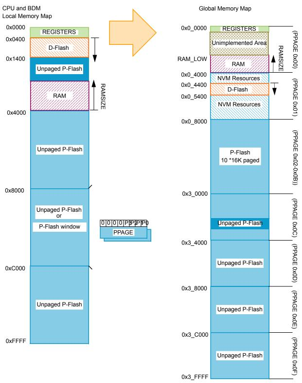
Figure 60. Local to global address mapping
