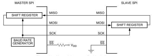
Figure 104. Master/slave transfer block diagram
