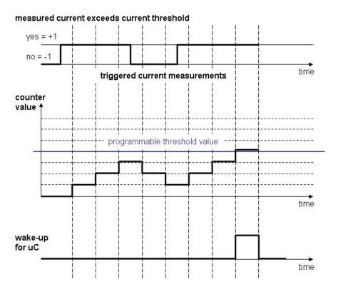
Figure 20. Current threshold - wake-up counter
