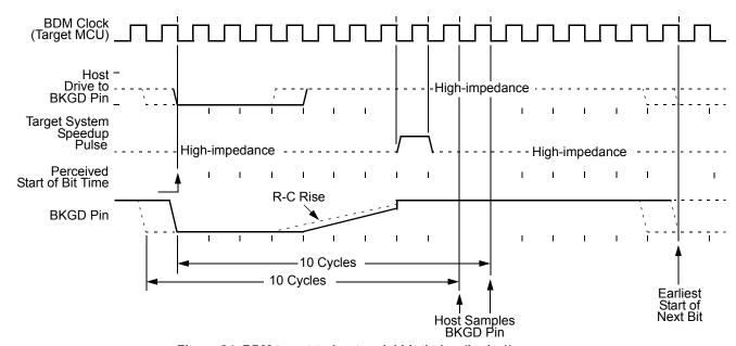
Figure 84. BDM target-to-host serial bit timing (logic 1)
