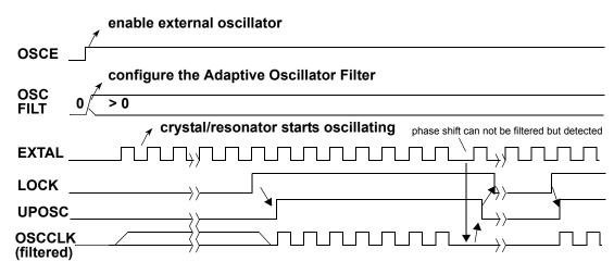
Figure 99. Critical noise detected by the adaptive oscillator filter
