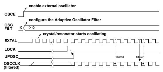
Figure 98. Noise filtered by the adaptive oscillator filter
