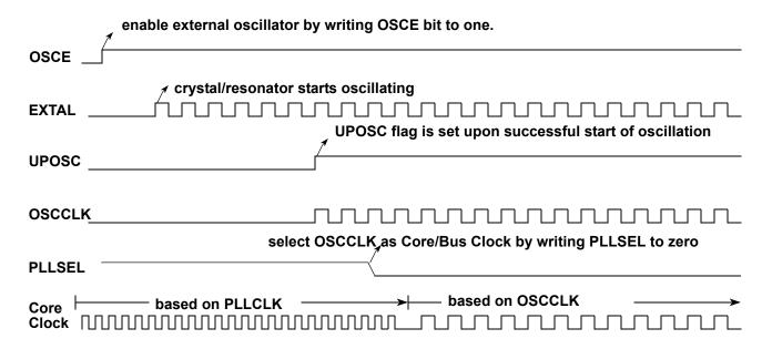
Figure 97. Enabling the external oscillator
