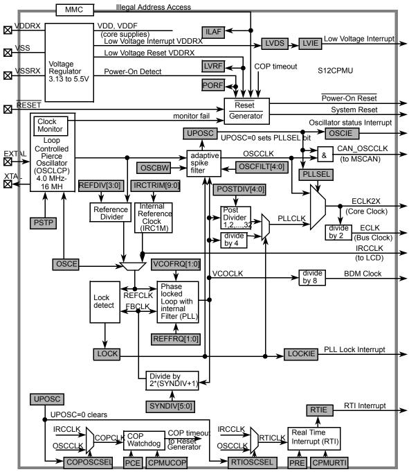
Figure 90. Block diagram of 9S12I128PIMV1
