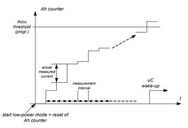
Figure 21. Ah counter function
