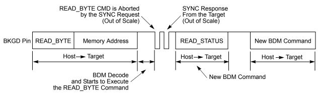
Figure 88. ACK abort procedure at the command level
