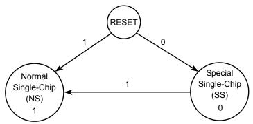
Figure 56. Mode transition diagram when MCU is unsecured
