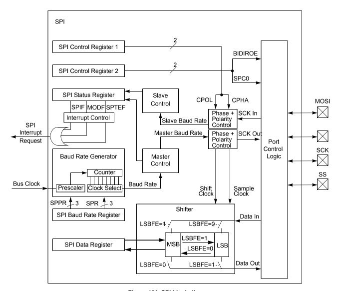
Figure 101. SPI block diagram
