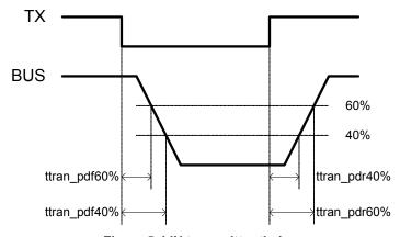
Figure 5. LIN transmitter timing
