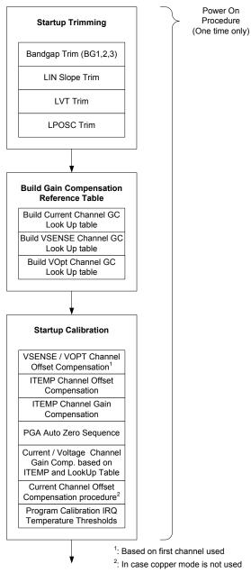
Figure 36. Power on procedure
