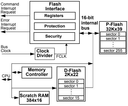
Figure 109. FTMRC128K1 block diagram
