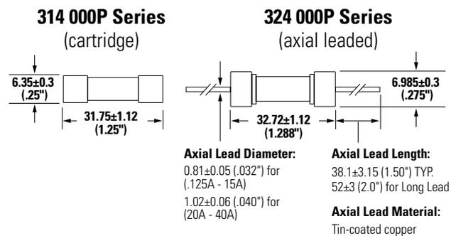
Measurements displayed in millimeters (inches)
