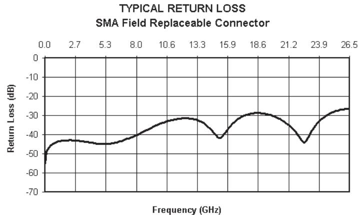
Although Johnson Components™ does not publish a VSWR specification for field replaceable connectors, typical connector VSWR can be expected to be less than  $1.1 + .01f$  ( $f$  in GHz). A VSWR specification is not stated because an industry standard method for testing field replaceable connectors does not exist. The actual performance of the connector is dependent upon the application for the following reasons:
