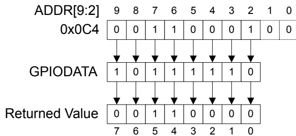
Figure 8-3. GPIODATA Read Example
