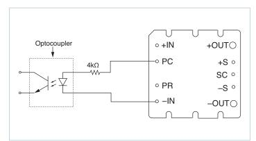
Figure 6 — Isolated on-state indicator
