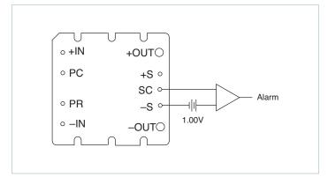
Figure 7 — Secondary-side on-state indicator
