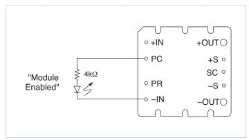
Figure 4 — LED on-state indicator
