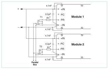
Figure 10 — Transformer-coupled interface
