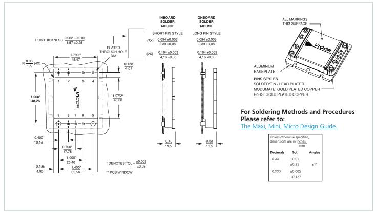
Figure 13 — PCB mounting specifications
