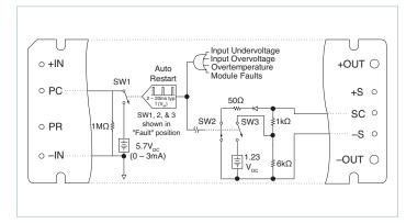
Figure 3 — PC/SC module alarm logic
