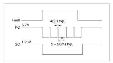
Figure 5 — PC/SC module alarm timing
