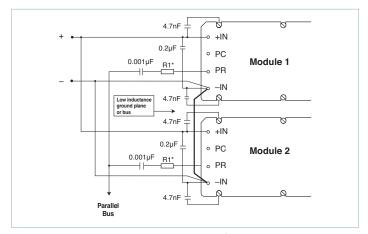
**Figure 9** — AC-coupled single-wire interface
