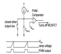
Figure 67. PWM circuit and timing diagram.
