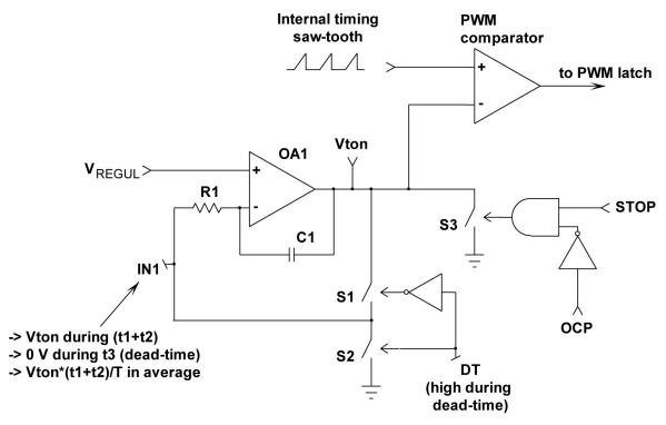
Figure 68. V<sub>TON</sub> Processing Circuit. The integrator OA1 amplifies the error between V<sub>REGUL</sub> and IN1 so that on average,  $(V_{TON} * (t_1+t_2)/T)$  equates V<sub>REGUL</sub>.
