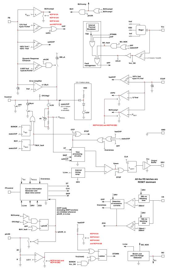
Figure 4. Block Diagram
