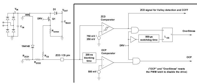
Figure 71. Current Sense and Zero Current Detection Blocks
