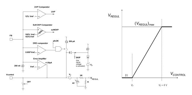
Figure 69. a) Regulation Block Figure (left), b) Correspondence between V<sub>CONTROL</sub> and V<sub>REGUL</sub> (right)
