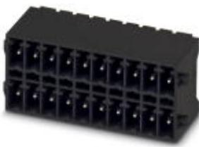
Header, Nominal current: 8 A, Rated voltage (III/2): 160 V, Number of positions: 15, Pitch: 3.5 mm, Color: black, Contact surface: Tin, Mounting: THR soldering, Article with engagement nose. The pin length is 14 mm. User information and design recommendations on Through Hole Reflow Technology can be found at: "Downloads"
