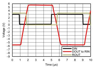
Figure 7. 250 kbps Driver to Receiver Loopback Timing Waveform,  $V_{CC}$ = 3.3 V
