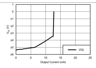
Figure 2. DOUT V<sub>OL</sub> vs Load Current, Both Drivers Loaded
