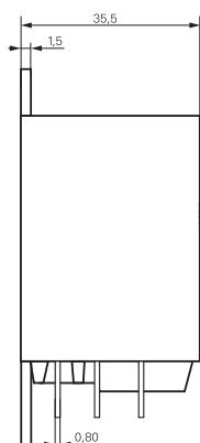
Cover with DIN-snap-on attachment (6.3mm quick connect only)
