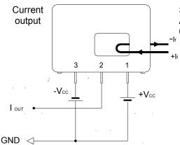
S26P200D15Y At  $I_f$  = 200A &  $V_{CC}$  = ±15 $V_{DC}$   $0\Omega \le R_M \le 56\Omega$
