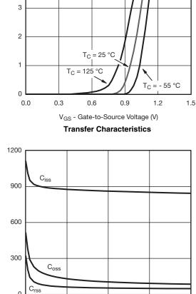
V<sub>DS</sub> - Drain-to-Source Voltage (V) Capacitance
