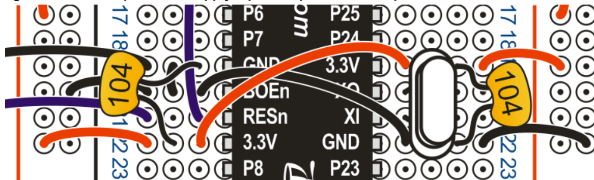
Figure 3-9: Close-up View of Supply Input Strap and Filter Capacitor Connections
