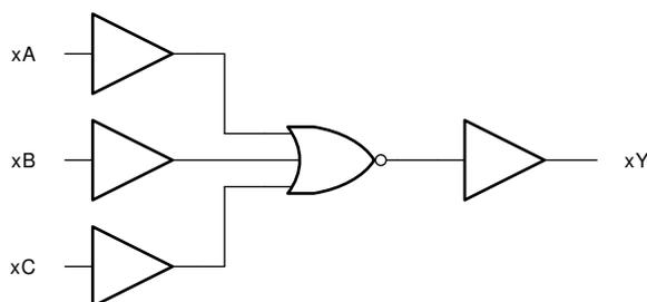
Figure 7-1. logic diagram, each gate (positive logic)
