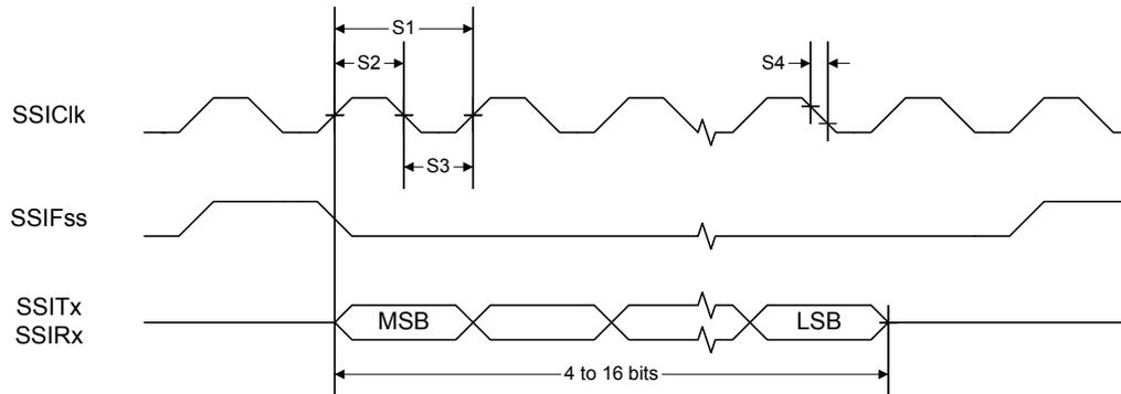
**Figure 23-15. SSI Timing for MICROWIRE Frame Format (FRF=10), Single Transfer**
