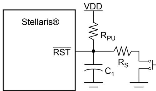
$$\text{Typical } R_{\text{PU}} = 10 \text{ k}\Omega$$
