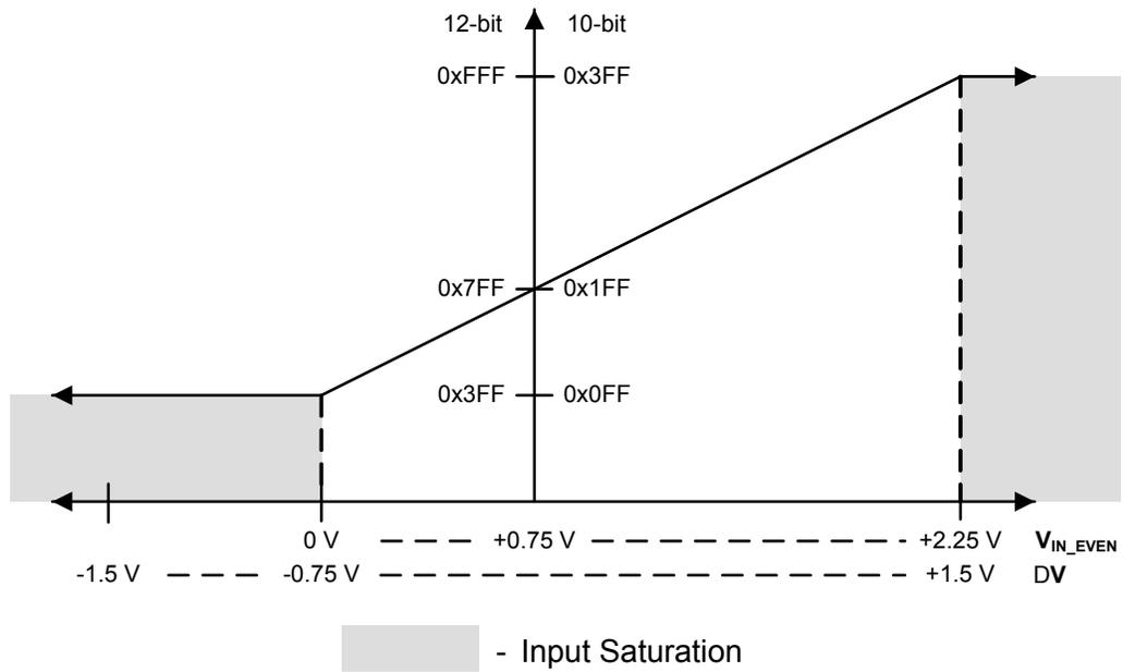
Figure 12-12. Differential Sampling Range,  $V_{IN\_ODD} = 2.25\text{ V}$
