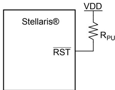
$R_{\text{PU}} = 0$  to 100 k $\Omega$
