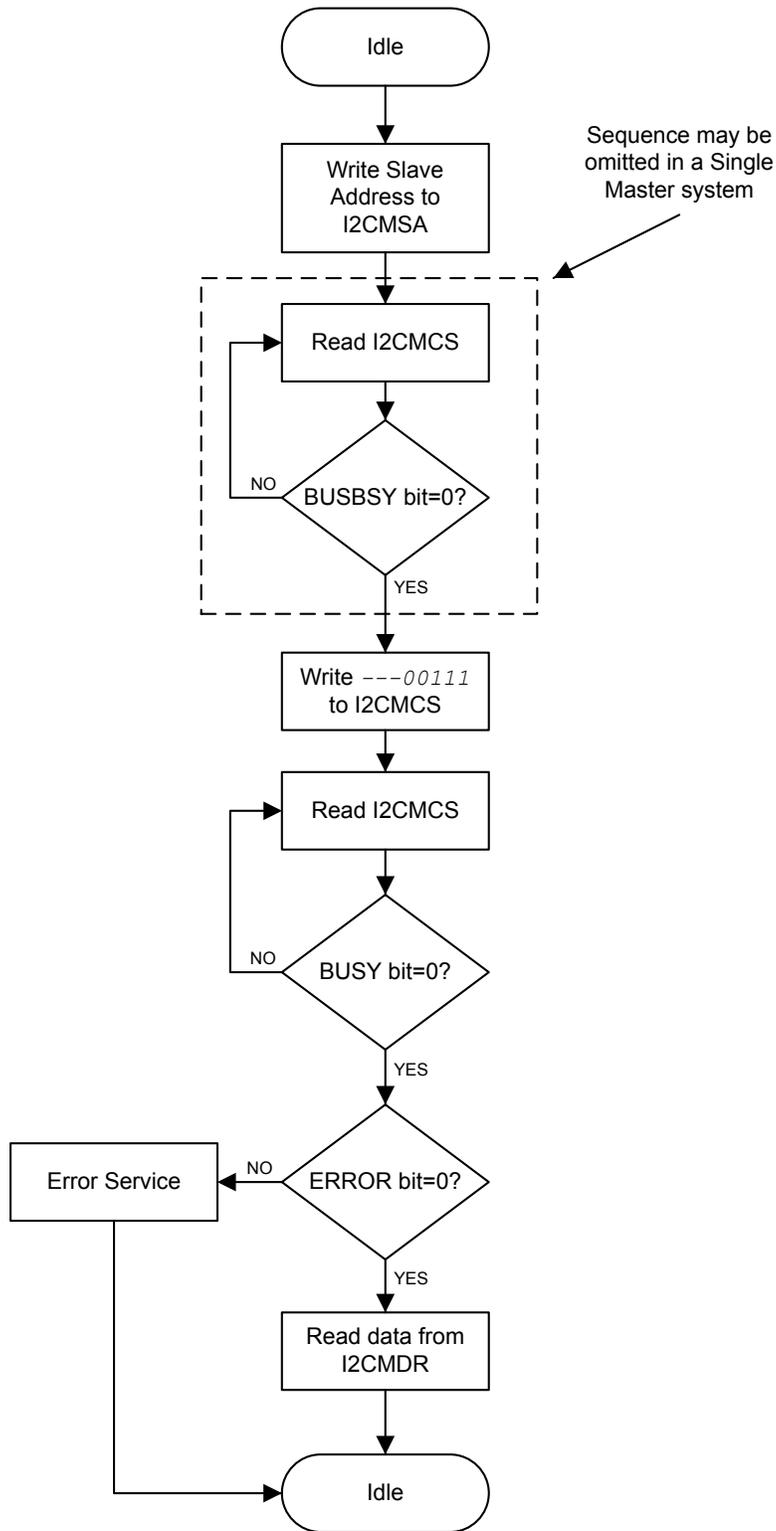
Figure 15-9. Master TRANSMIT with Repeated START
