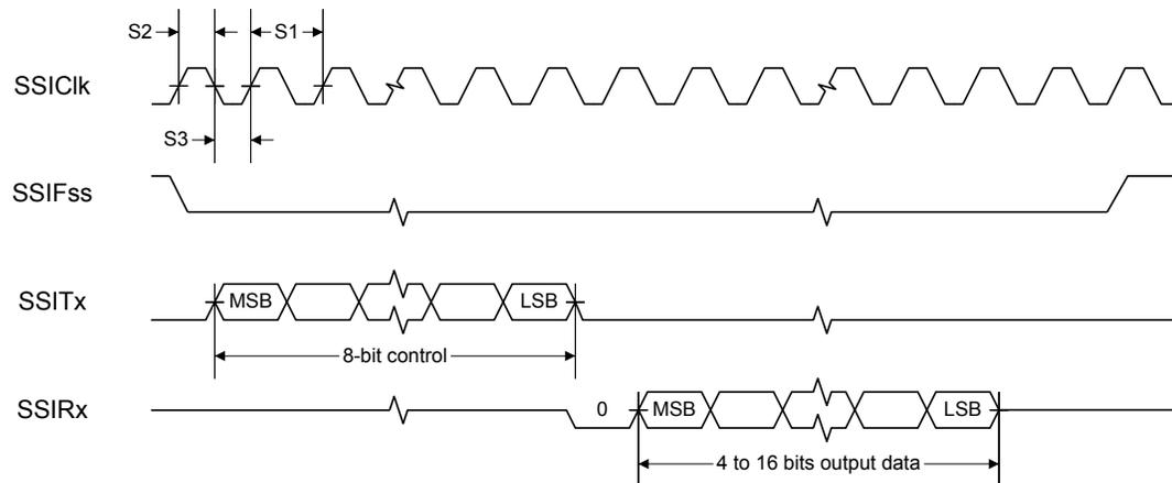
Figure 23-16. SSI Timing for SPI Frame Format (FRF=00), with SPH=1
