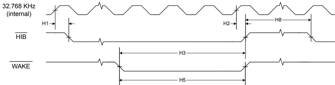
**Figure 23-12. Hibernation Module Timing with Internal Oscillator Stopped in Hibernation**
