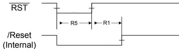
Figure 23-8. Software Reset Timing
