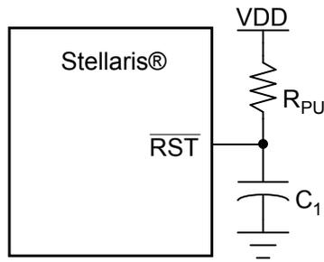
$$R_{\text{PU}} = 1 \text{ k}\Omega \text{ to } 100 \text{ k}\Omega$$
