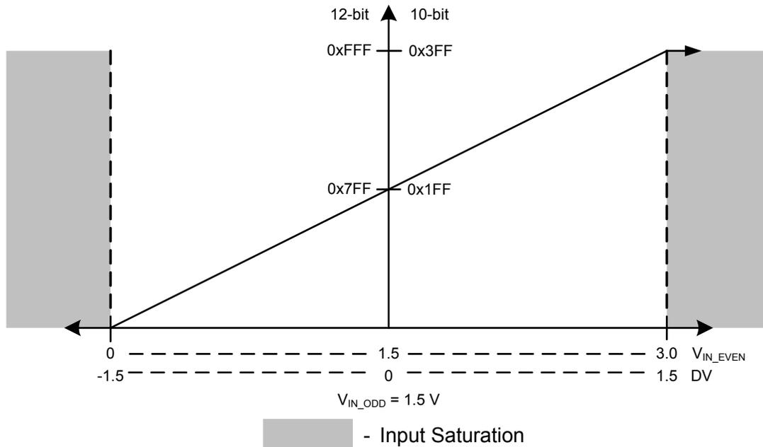
Figure 12-11. Differential Sampling Range,  $V_{IN\_ODD} = 0.75\text{ V}$
