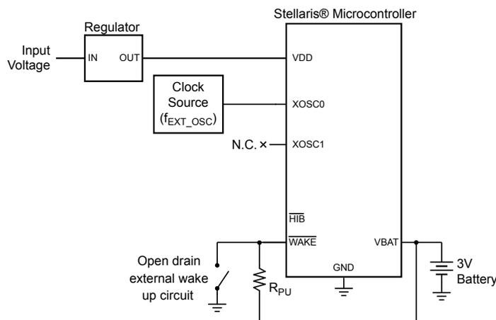
**Note:**  $R_{PU}$  = Pull-up resistor is 1 M $\Omega$
