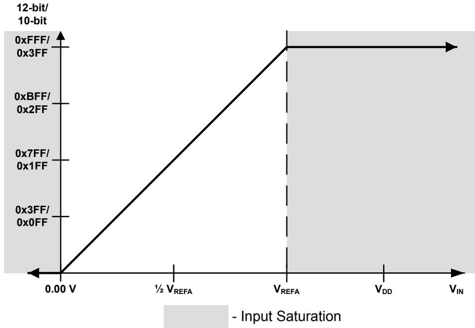
Figure 12-9. External Voltage Conversion Result with 1.0-V Setting
