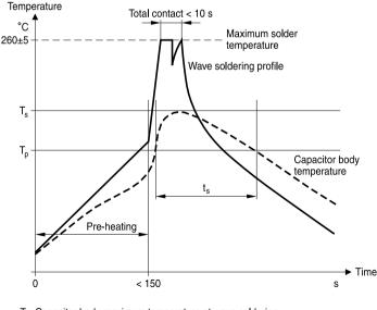
Ts: Capacitor body maximum temperature at wave soldering
