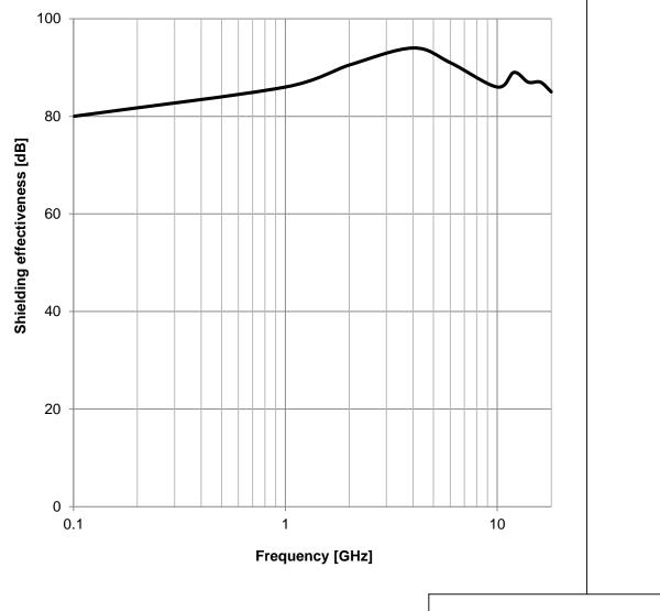
CHECKED REVISION DATE (YYYY-MM-DD) GENERAL TOLERANCE PROJECTION METHOD ViMa 005.003 2020-03-06 DIN ISO 2768-1m DESCRIPTION **WE-LT Conductive Shielding** Würth Elektronik eiSos GmbH & Co. KG Gasket ORDER CODE EMC & Inductive Solutions Max-Eyth-Str. 1 3020701 74638 Waldenburg Germany SIZE/TYPE STATUS Tel. +49 (0) 79 42 945 - 0 www.we-online.com BUSINESS UNIT PAGE WÜRTH ELEKTRONIK 2/3 eiSos Valid Square eiSos@we-online.com
