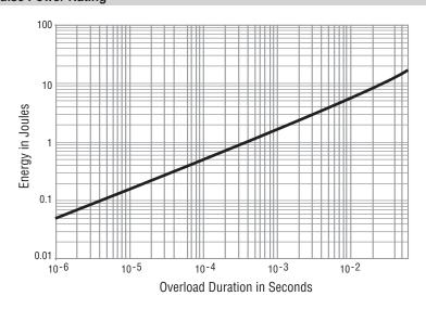
The energy absorbed by the resistor expressed in Joules can be calculated by multiplying the peak power of the pulse in watts times the length of the pulse in seconds.
