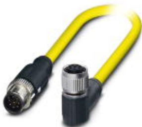
Sensor/actuator cable, 8-position, PVC, yellow, shielded, Plug straight M12 SPEEDCON, coding: A, on Socket angled M12 SPEEDCON, coding: A, cable length: 1.5 m
