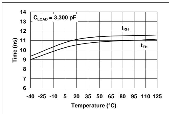
**FIGURE 2-2:** HIGHDR Rise and Fall Time vs. Temperature.
