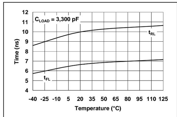
**FIGURE 2-5:** LOWDR Rise and Fall Time vs. Temperature.
