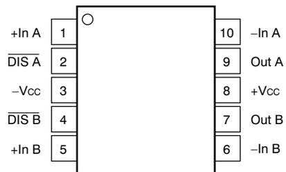
**Figure 1. MSOP Package Pinout, Top View**
