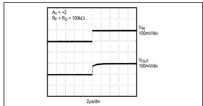
Figure 2b. Pulse Response with  $10\text{pF}$  Feed-Forward Compensation
