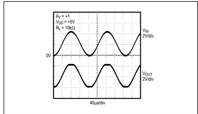
Figure 3. Overdriven Input Showing No Phase Reversal
