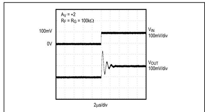
Figure 2a. Pulse Response with No Feed-Forward Compensation
