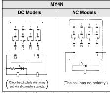
An AC model has coil disconnection self-
