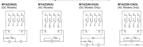
Note: For the DC models, check the coil polarity when wiring and wire all connections correctly.
