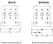
Check the coil polarity when wiring and wire all connections correctly.
