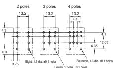
The dimensional tolerance is  $\pm 0.1$ . Refer to the terminal arrangement and internal connections diagrams for the MY2, MY3, MY4, and MY4Z.
