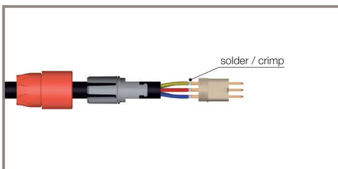
4. Slide the collet ② forward and locate both tags ③ in the slots ⑤ on the insulator ⑥.
