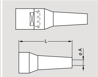
A bend relief absorbs the angular force that may be exerted on cables.
