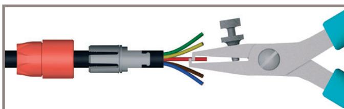
2. Strip the cable according to the lengths given in the table.
