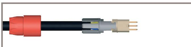
5. Slide collet nut ① over collet ② and tighten the collet nut ① to the maximum torque of 0.3 Nm.
