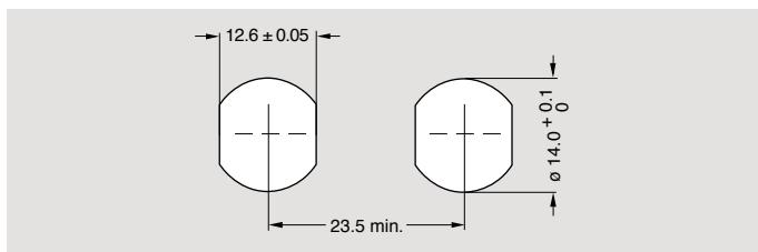
**Note:** Socket mounting nut torque = 1 Nm.
