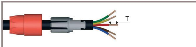
3. Solder conductors into contacts, starting with the center conductor, making sure that neither solder nor flux gets onto the insulator or cable insulation.
