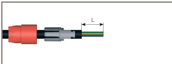
1. Slide the collet nut ① and then the collet ② onto the cable.
