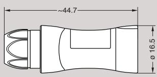
**SRN** Free socket, key (N) or keys (P, S and T), with cable collet and nut for fitting a bend relief
