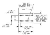
N SOLDER PINS WITH .100" SPACING
