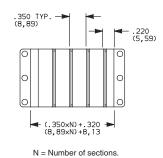
SWITCH SECTION ONLY-UNASSEMBLED WITHOUT ENDPLATES OR SPACERS (Must be ordered with number of sections option "0", see Page M-4.)
