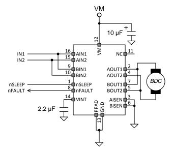
Figure 9. Parallel Mode Schematic
