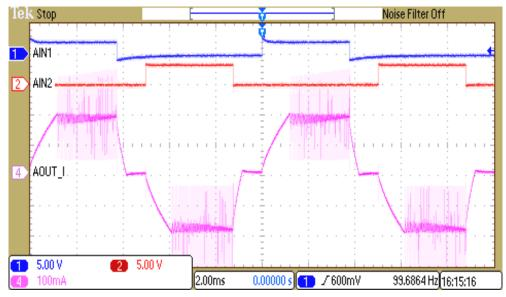
A. Channel 1 is the AIN1 input PWM signal, and channel 2 is the AIN2 input PWM signal. BIN1 and BIN2 follow the same pattern, but are shifted by 90° from AIN1 and AIN2 as shown in Figure 11. Channel 4 is the output current in the direction AOUT1 → AOUT2. In forward and reverse drive, the current rises until it hits the current chopping limit of 200 mA, and is regulated at that level with fixed-off time current chopping.
