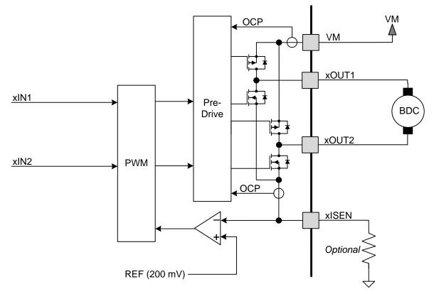
Figure 6. H-Bridge and Current-Chopping Circuitry
