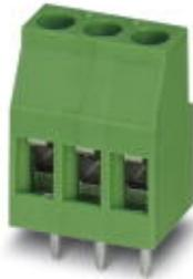
PCB terminal block, nominal current: 24 A, nom. voltage: 400 V, pitch: 5.08 mm, number of positions: 3, connection method: Screw connection with tension sleeve, mounting: Wave soldering, conductor/PCB connection direction: 0 °, color: black. The article can be aligned to create different nos. of positions!
