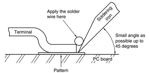
4) Be aware that soldering while applying a load on the connector terminals may cause improper operation of the connector.
