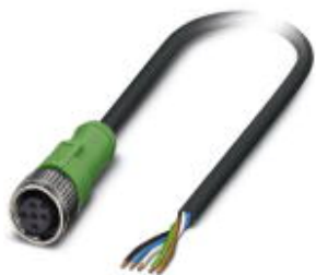
Sensor/actuator cable, 5-position, PVC, black RAL 9005, free cable end, on Socket straight M12, A - standard, cable length: 5 m
