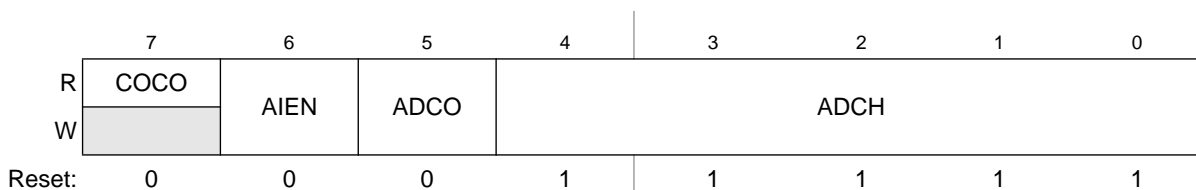
Figure 10-3. Status and Control Register (ADCSC1)
