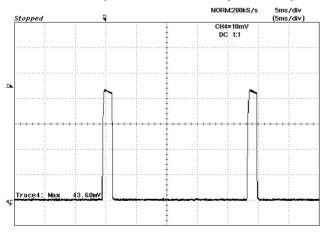
Figure 27: Output short circuit current 5Vin, 0.75Vout
