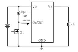
Figure 35: Negative remote On/Off implementation
