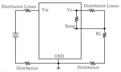
Figure 36: Effective circuit configuration for remote sense operation
