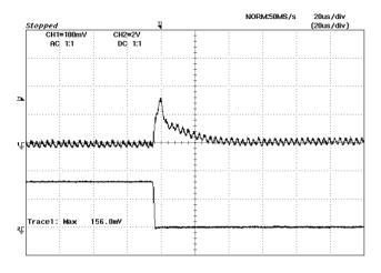
Figure 19: Typical transient response to step load change at 2.5A/ $\mu$ S from 100% to 50% of lo, max at 5Vin, 3.3Vout (Cout = 1 $\mu$ F ceramic, 10 $\mu$ F tantalum)
