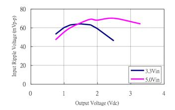
Figure 33: Input voltage ripple for various output models, Io = 6A (CIN = 4×100µF tantalum // 2×47µF ceramic)
