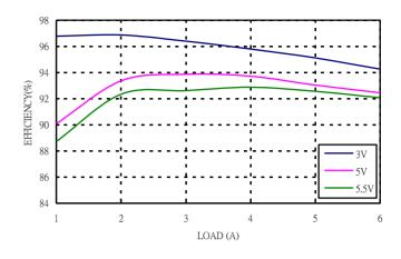
Figure 2: Converter efficiency vs. output current (2.5V out)
