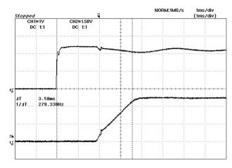
Figure 11: Turn on delay time at 3.3Vin, 2.5V/6A out
