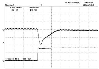
**Figure 24:** Typical transient response to step load change at 2.5A/μS from 50% to 100% of lo, max at 3.3Vin, 2.5Vout (Cout =1uF ceramic, 10μF tantalum)
