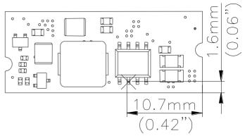
Figure 44: Temperature measurement location The allowed maximum hot spot temperature is defined at 127  $\mathcal{C}$
