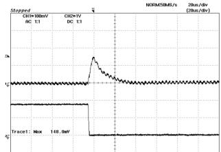
**Figure 25:** Typical transient response to step load change at 2.5A/μS from 100% to 50% of lo, max at 3.3Vin, 1.8Vout (Cout =1uF ceramic, 10μF tantalum)
