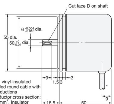
\*5-dia. vinyl-insulated shielded round cable with 5 conductors (Conductor cross section: 0.18 mm<sup>2</sup>, Insulator diameter: 1.1 mm), Standard length: 500 mm
