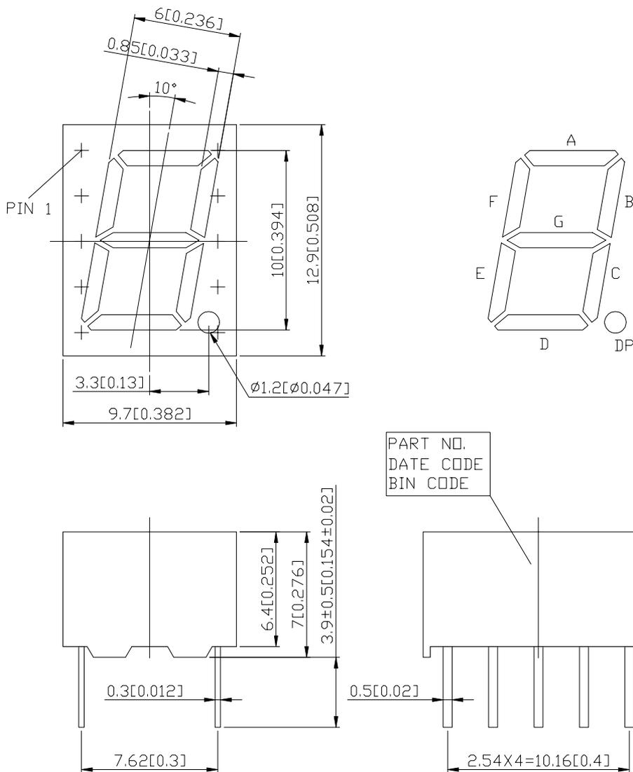
NOTES: All dimensions are in millimeters. Tolerance is  $\pm 0.25$ -mm (0.01") unless otherwise noted.
