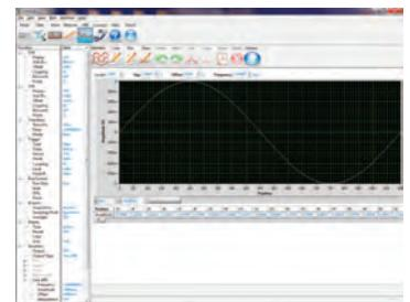
Generate, edit, and upload arbitrary waveforms to the scope using the intuitive Comsoft PC software.
