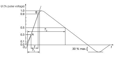
$\begin{array}{ll} \mbox{Front time:} & T_1 = 1.67 \mbox{ x } T = 1.2 \mbox{ } \mu s \pm 30 \mbox{ } \% \\ \mbox{Time to half-value:} & T_2 = 50 \mbox{ } \mu s \pm 20 \mbox{ } \% \\ \end{array}$
