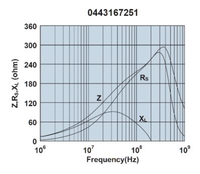
Impedance, reactance, and resistance vs. frequency.
