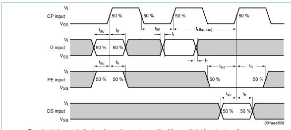
The shaded areas indicate where change is permitted for predictable output performance. Set-up and hold times are shown as positive values but may be specified as negative values. Measurement points are given in Table 9.
