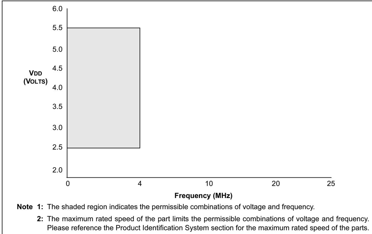
**FIGURE 12-10: PIC16C620A/C621A/C622A/CR620A - 40 VOLTAGE-FREQUENCY GRAPH,  $0^{\circ}\text{C} \leq T_A \leq +70^{\circ}\text{C}$**
