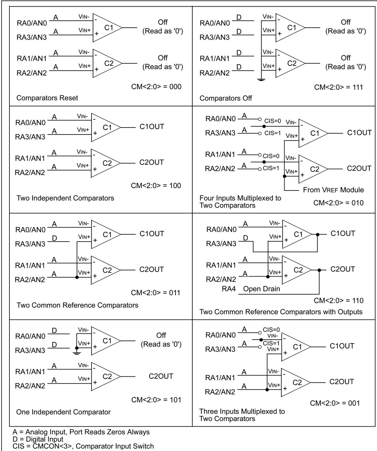
The code example in Example 7-1 depicts the steps required to configure the comparator module. RA3 and RA4 are configured as digital output. RA0 and RA1 are configured as the V- inputs and RA2 as the V+ input to both comparators.
