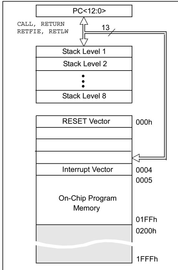
**FIGURE 4-2: PROGRAM MEMORY MAP AND STACK FOR THE PIC16C621/PIC16C621A**
