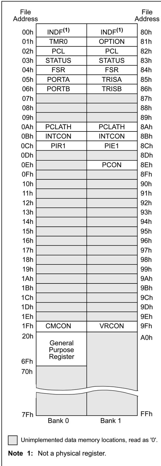
**FIGURE 4-5: DATA MEMORY MAP FOR THE PIC16C622**
