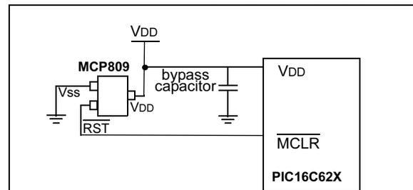
This brown-out protection circuit employs Microchip Technology's MCP809 microcontroller supervisor. The MCP8XX and MCP1XX families of supervisors provide push-pull and open collector outputs with both high and low active RESET pins. There are 7 different trip point selections to accommodate 5V and 3V systems.
