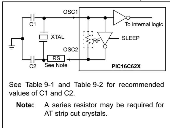
**FIGURE 9-2: EXTERNAL CLOCK INPUT OPERATION (HS, XT OR LP OSC CONFIGURATION)**
