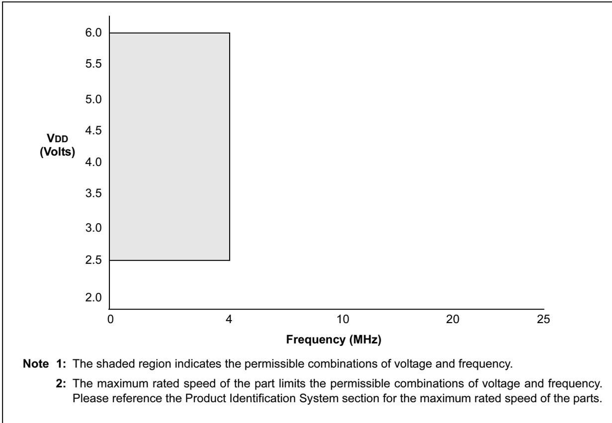
**FIGURE 12-3: PIC16C62XA VOLTAGE-FREQUENCY GRAPH,  $0^{\circ}\text{C} \leq T_A \leq +70^{\circ}\text{C}$**
