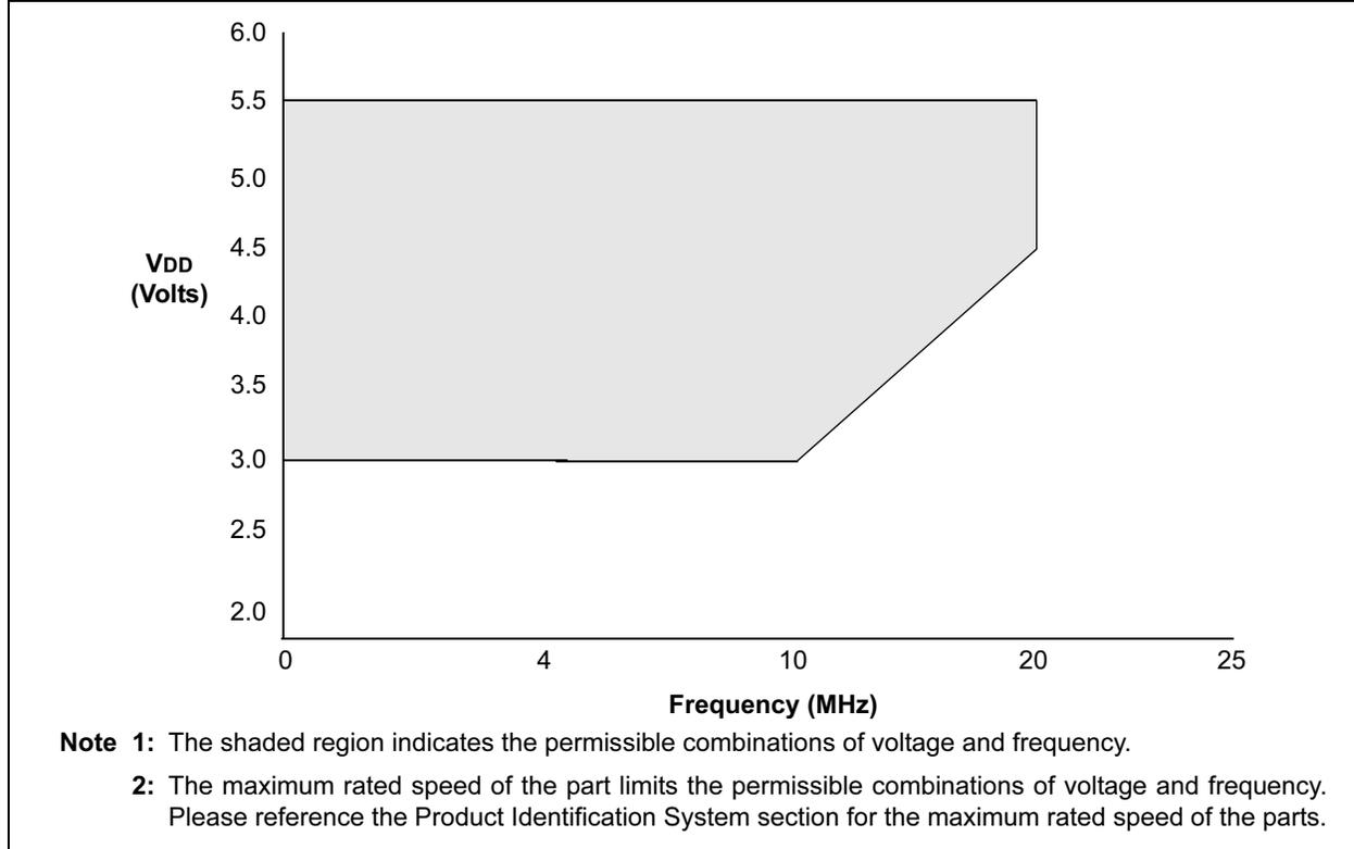
**FIGURE 12-8: PIC16CR62XA VOLTAGE-FREQUENCY GRAPH,  $-40^{\circ}\text{C} \leq T_A \leq 0^{\circ}\text{C}$ ,  $+70^{\circ}\text{C} \leq T_A \leq +125^{\circ}\text{C}$**
