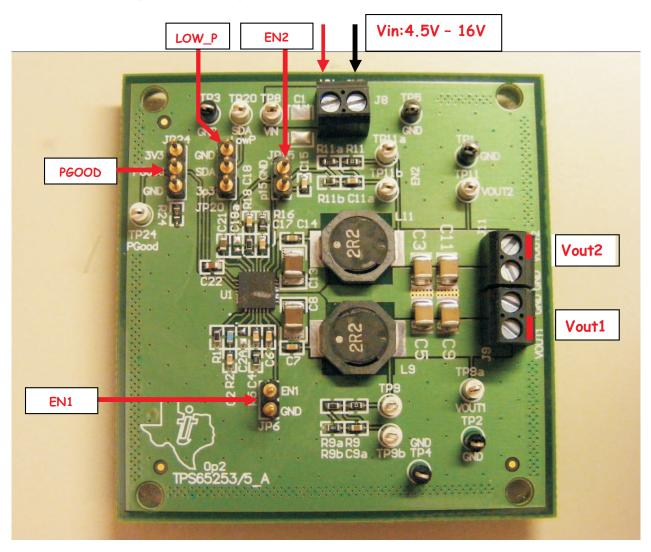
Figure 7. Headers Description and Jumper Placement
