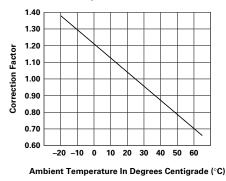
To use this chart: Read up from the ambient temperature to the curve, and across to find a correction factor. Multiply the breaker rating by the correction factor to determine the compensated rating. Calculate the overloads in terms of the compensated rating to use the published trip curve.
