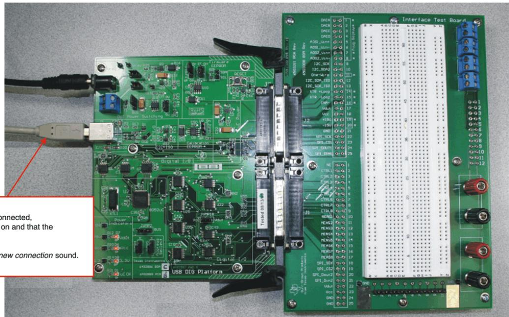
The first time a USB DIG board is connected, be sure that the PC sound is turned on and that the power supply is first connected. Then plug in the USB cable. You should hear a typical Windows *new connection* sound.
