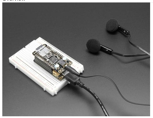
Bend all audio files to your will with the Adafruit Music Maker FeatherWing! It's a fun-size version of our Music Maker shield for Arduino (https://adafru.it/tbM)! This powerful shield features the VS1053, an encoding/decoding (codec) chip that can decode a wide variety of audio formats such as MP3, AAC, Ogg Vorbis, WMA, MIDI, FLAC, WAV (PCM and ADPCM). You can do all sorts of stuff with the audio as well such as adjusting bass, treble, and volume digitally.
