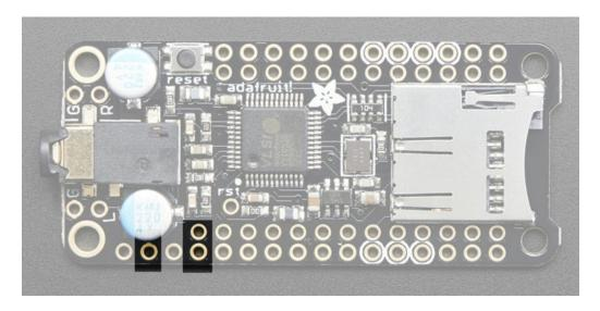
For both headphone & amp version: to power the SD card and MP3 chip, we need power from the **3V** (2nd pin) and **GND** (4th pair of pins).
