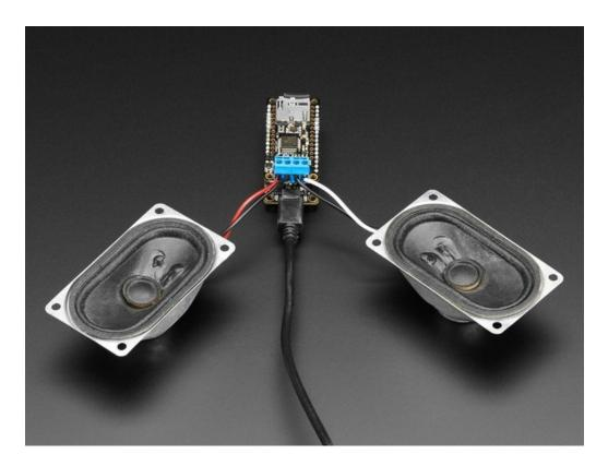
All this functionality is implemented in a light-weight SPI interface so that any Feather Board can play audio from an SD card. There's also a special MIDI mode that you can boot the chip into that will read 'classic' 31250Kbaud MIDI data from the UART TX pin and act like a synth/drum machine - there are dozens of built-in drum and sample effects!
