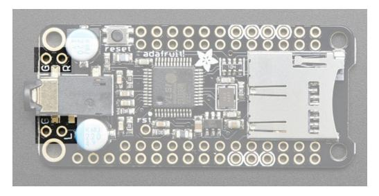
If you don't want to use a 3.5mm jack, you can always connect directly to the **Ground, Right** and **Left** pins next to the headphone jack. They are line level, AC coupled outputs - so its safe to connect them to an amplifier or other device input.
