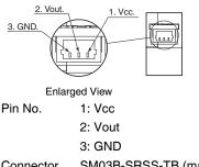
Connector SM03B-SRSS-TB (made by J.S.T. Mfg. Co.)
