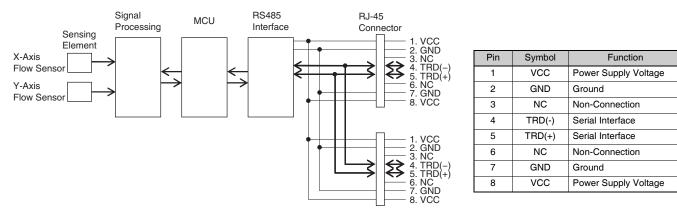
The sensor has two port of RJ-45 connectors (8 pins), and all the pair of each pin is connected internally. These connectors can be used for daisy chain wiring when using multiple devices on the same bus (multi-drop connection).
