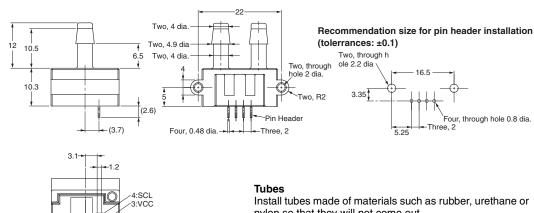
nylon so that they will not come out. For urethane tubes, tubes with an outer diameter of 6 mm and an inner diameter of 4 mm are recommended.
