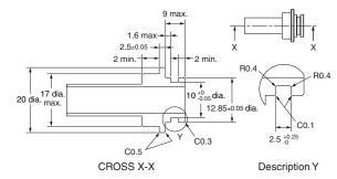
If using a Rc3/8 converter joint, the following is recommended. REGAL JOINT CO., LTD eigyou@rgl.co.jp Converter male joint (Rc3/8-Quick male joint): Adapter Rc3/8-QJM10 O ring: O ring P10 fluororubber (material)
