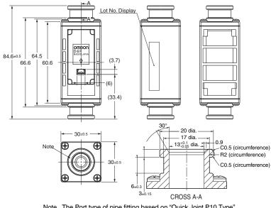
Note. The Port type of pipe fitting based on "Quick Joint P10 Type". \* P10 shows the name of an O-ring prescribed by JIS B 2401.
