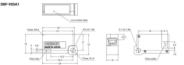
D6F-D MEMS 2-Axis Flow Sensor
