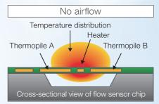
During the absence of airflow, the temperature distribution around the heater is symmetrical. When there is airflow, the temperature of the upwind side cools down and the temperature of the downwind side warms up, disrupting the symmetry of the temperature distribution.
