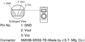
Use the following connectors made by J.S.T. Mfg. Co. for connections to the Sensor:
