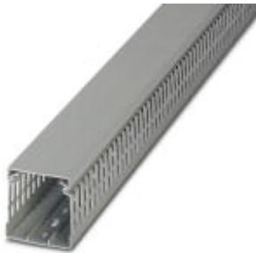
Cable duct, light gray, halogen-free, consisting of upper part and mounting base, width: 120 mm, height: 80 mm, length: 2000 mm
