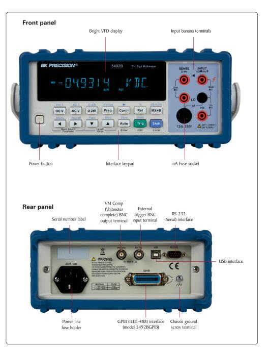
True RMS Bench Multimeter Model 5492B
