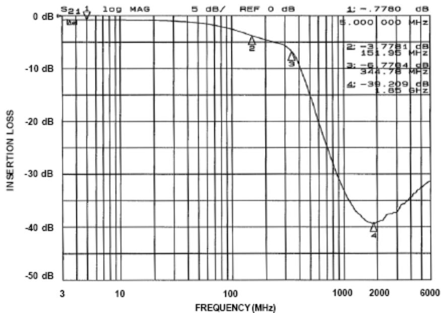
Figure 4. Insertional Loss vs. Frequency (Filter 4: CM1452-04, -06, -08)
