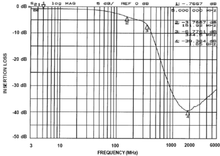
Figure 5. Insertional Loss vs. Frequency (Filter 5: CM1452-06, -08)
