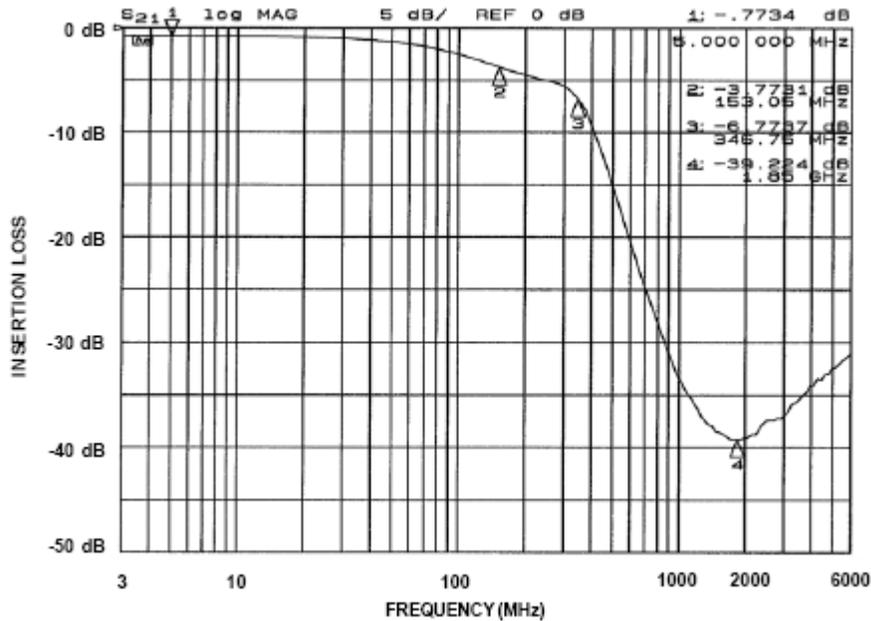
Figure 8. Insertional Loss vs. Frequency (Filter 8: CM1452-08)
