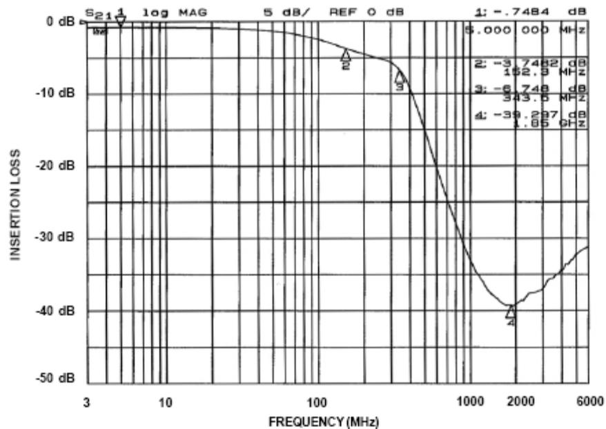
Figure 2. Insertional Loss vs. Frequency (Filter 2: CM1452-04, -06, -08)
