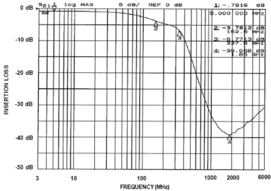
Figure 1. Insertional Loss vs. Frequency (Filter 1: CM1452-04, -06, -08)
