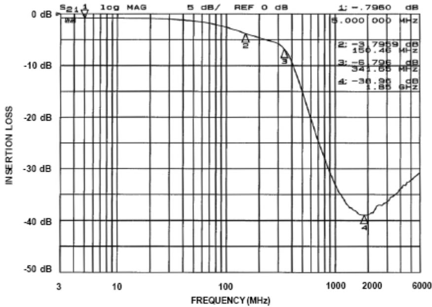
Figure 3. Insertional Loss vs. Frequency (Filter 3: CM1452-04, -06, -08)
