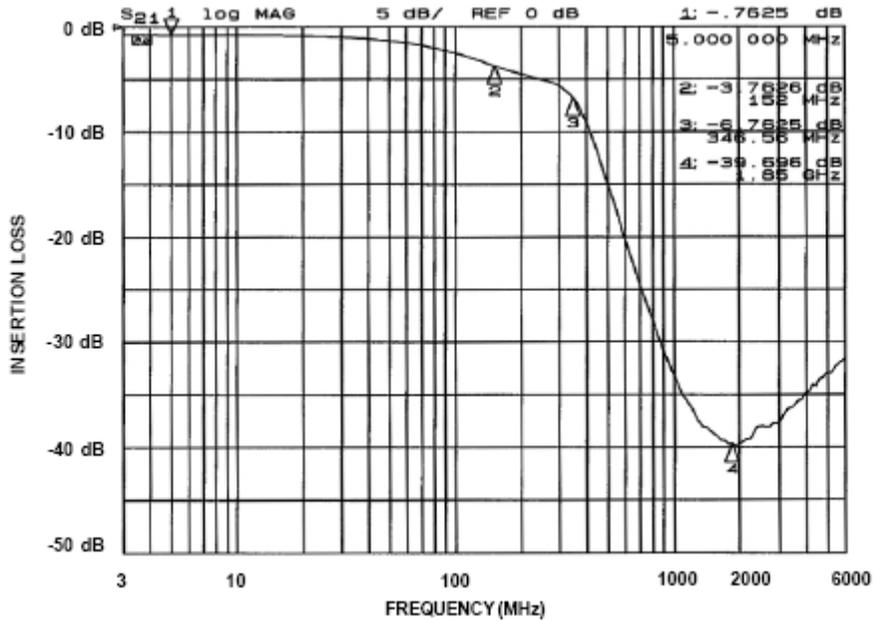
Figure 7. Insertional Loss vs. Frequency (Filter 7: CM1452-08)
