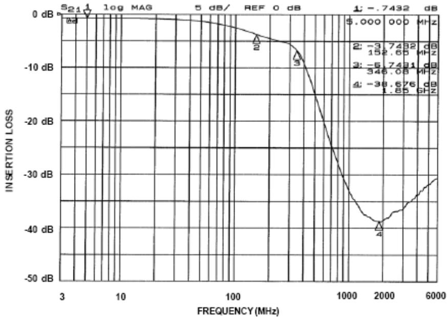
Figure 6. Insertional Loss vs. Frequency (Filter 6: CM1452-06, -08)
